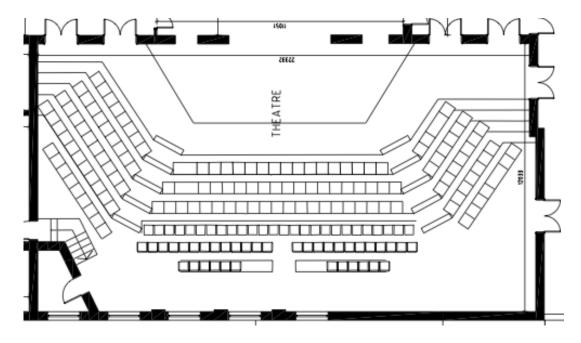
The main playing area is the thrust beyond the proscenium. This area is 3.7m in depth, 12.5m wide upstage and 8.02m wide downstage. There are two additional onstage entrances. The proscenium and these two entrances can be left open or closed with existing curtains (black).
